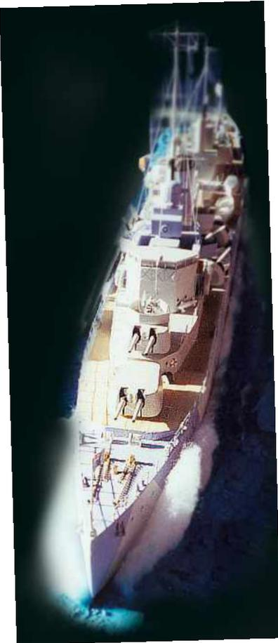
**Know your ship. From a model of Achilles... Left the deck from for'd showing A and B turrets. Some of the 5 inch AA turrets can be seen too. Right Looking from aft X and Y turrets. X turret is traditionally manned by Royal Marines.. Five inch AA turrets and torpedo tubes can be made out as well as the crane for the seaplane.**
